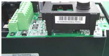
The condition that two places of nails of NES1-OPE were off.
