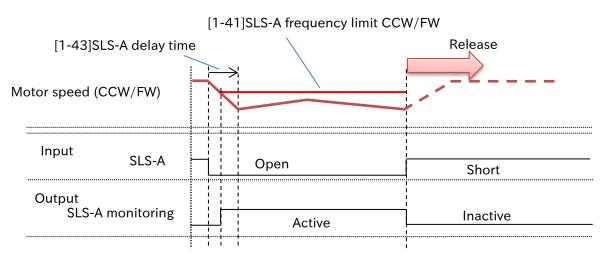
e.g. Case: SLS-A activating when the motor speed is under frequency limit and driving CW/RV:
