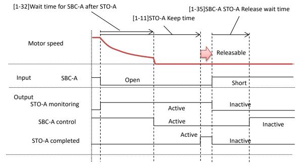
e.g. Case: SBC-A activating before STO-A activating [1-31]SBC-A Time linkage=01(SBC before STO), [1-12]STO-A Release mode =01(With safety signal) and [1-36]SBC-A release level=0.00%:
