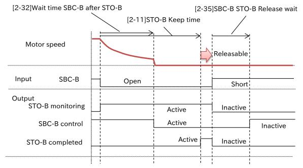
e.g. Case: SBC-B activating before STO-B activating [2-31]SBC-B Time linkage=01(SBC before STO), [2-12]STO-B release mode=01(With safety signal) and [2-36]SBC-B release level=0.00%:
