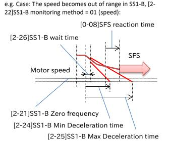
[0-08]SFS reaction time Motor speed [2-21]SDI-B Zero frequency SFS
