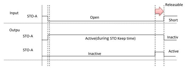
e.g. [1-12]STO-A Release Mode =02(With release signal):
