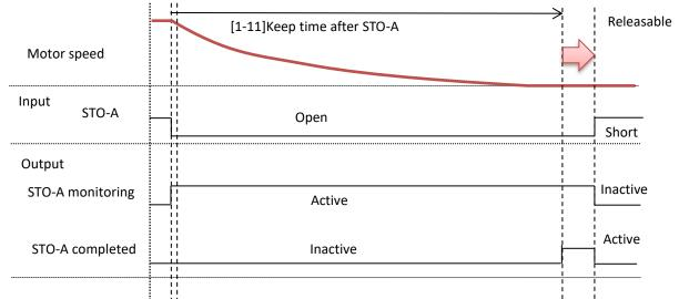
e.g. Case: [1-12]STO-A release mode = 02 (With release signal):
