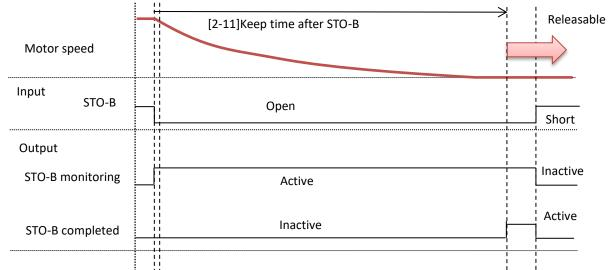
e.g. Case: [2-12]STO-B release mode = 02 (With release signal):
