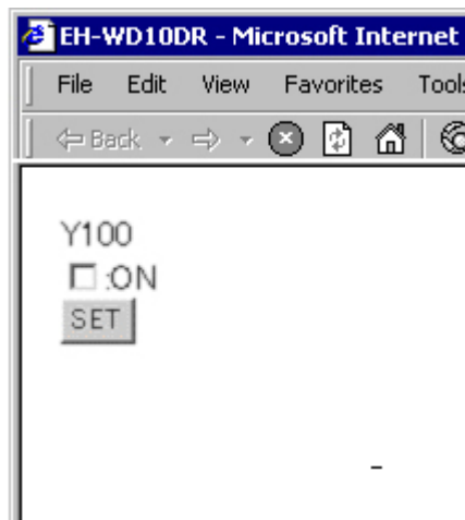
Figure 15.8 HTML tag example (5) for data memory setting
