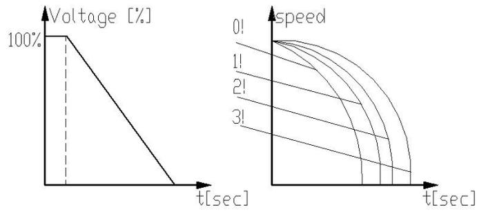
**Curve 4 - Torque Curve** - Provides linear deceleration of the torque. In certain loads, linear torque deceleration can result in close to linear speed deceleration. The RVS-DXM Torque Control does not require any external torque or speed sensor (tacho-gen. etc.).
