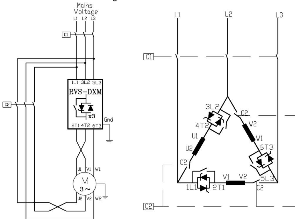
Reverse speed with RVS-DXM connected INSIDE DELTA.
