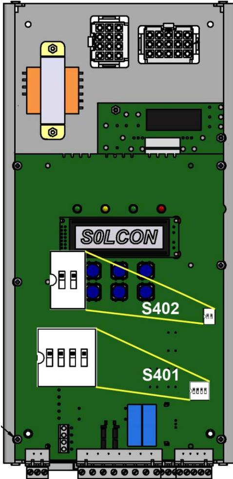
5. Set the dip switches according to the below table:
