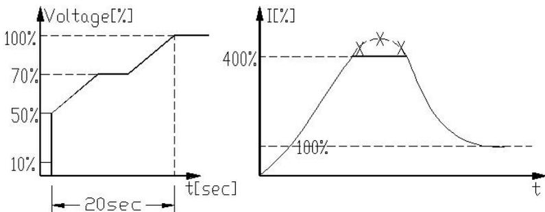
Voltage and current increase until current reaches CURRENT LIMIT. The voltage is held at this value until motor is close to nominal speed, then current will begin to decrease. The RVS-DXM continues to ramp-up the voltage until reaching nominal. Motor speed smoothly accelerates to full speed.
