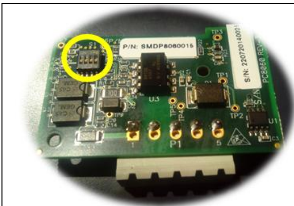
Figure 8: Location of the dip switches on the Thermistor In and Analog Out option card
